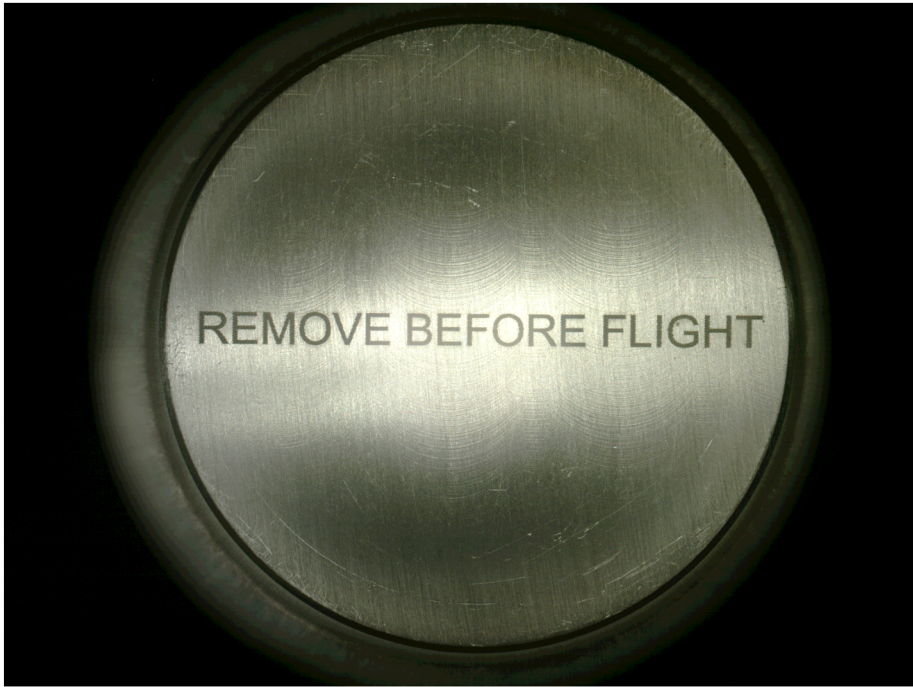
Fig. 38 Flight Cachecam image acquired during ATLO testing. The remove-before-flight cover shown in this image has a diameter of approximately 46.4 mm. The spatial scale of this image is approximately 12.5 microns/pixel (the cover is not exactly at the best focus distance)
