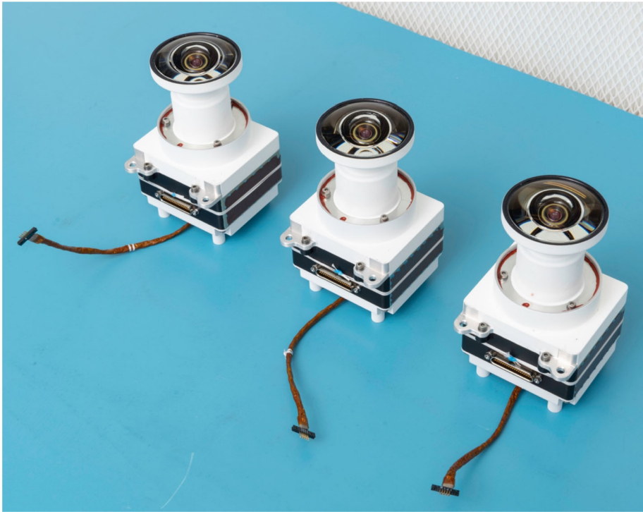
Fig. 13 Flight Hazcam cameras
